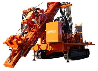
Small enough to be shipped in a 20' shipping container, the SDC-375 comes track-mounted or in a truck-mount configuration, if required, and fully supported by Sonic Drill Corporation's industry-standard one year warranty. For its under \$500,000 price tag, the machine also comes fully-optioned and work ready with one week of operator training included.
