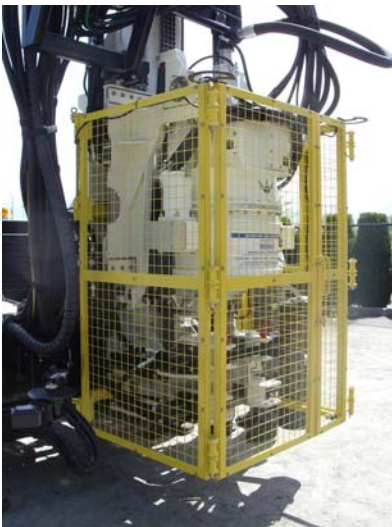
Sonic Drill Corporation displays its new drill head safety cage.
