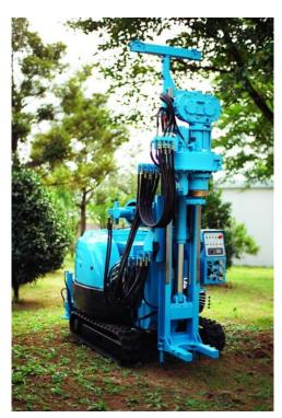
Like its larger twin, the Sonic Probe works by forcing oscillations down the drill string to allow it to easily buzz through a variety of materials – with or without using any drilling fluid and without producing any cuttings. And, thanks to its distinctive drilling method, bylaw officers and neighbors will be kept at bay by its quiet hum.
